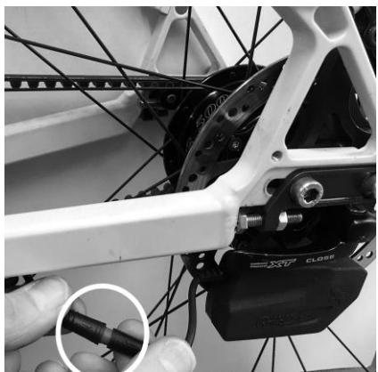
Re-connect the Rohloff E-14 Shifter Unit with the Bosch eBike System cable loom.
