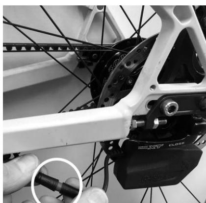
Disconnect the cable from the Rohloff E-14 Shifter Unit on the rear wheel.
