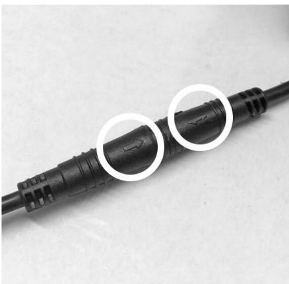
Both cable plugs are embossed with an arrow indicating their correct orientation.
